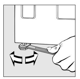
The screw feet can be adjusted to compensate for any uneveness in the floor surface.
